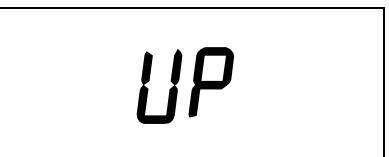
14. And press
